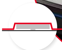
Profile membrane keypads Height: approx. 1.0 - 1.5 mm*
